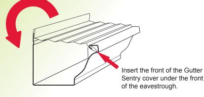
Note that the Gutter Sentry directly snaps over the back of the gutter; no crimping is required to maintain it in place.
