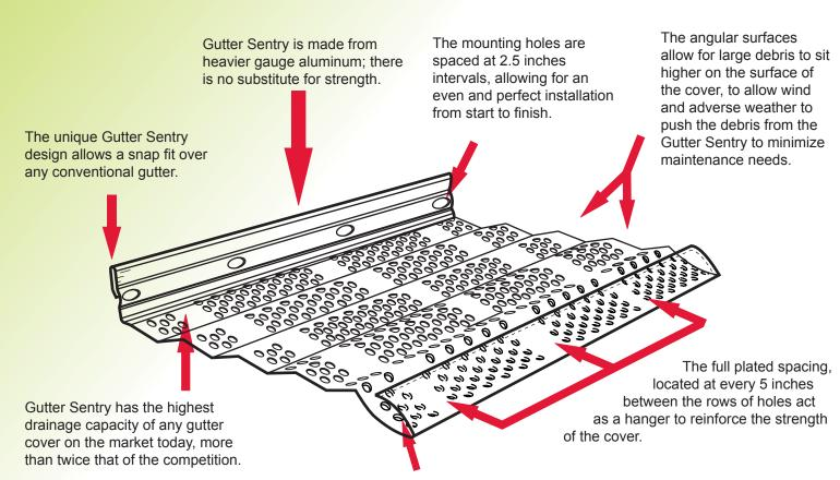
The unique and patented "football" design allows Gutter Sentry to fit over any lip easily and efficiently. The drainage holes within the "football" allow for continued drainage.
